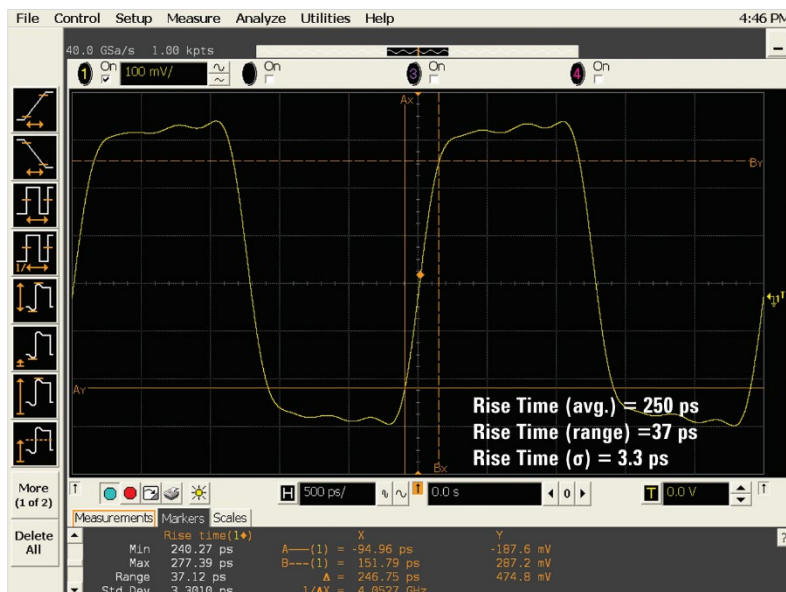
Figure 15a. 400 MHz clock captured on a Keysight Infiniium 3 GHz oscilloscope sampling at 40 GSa/s.
