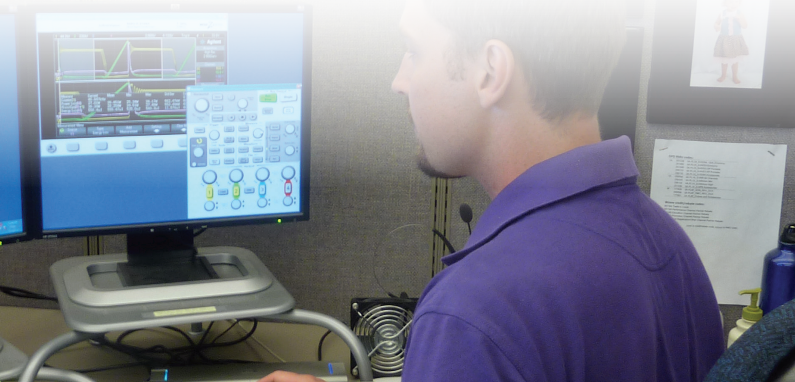
Figure 29. The built-in web browser of Keysight's InfiniiVision, with a virtual remote front-panel user interface, makes it easy to control and access "live" oscilloscope measurements from anywhere in the world
