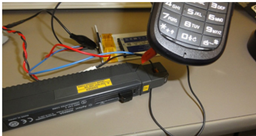
Figure 4-2. A simple way to measure a current with an oscilloscope is to use a clamp-on type current probe such as Keysight's 1147B or N2893A.
